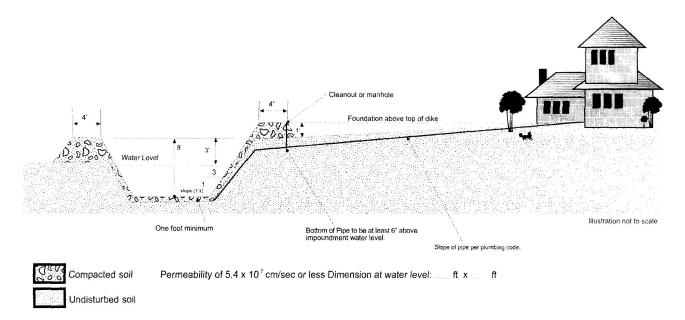
When using this chart to size a rectangular impoundment, calculate the area of a square impoundment and then modify the length and width of the sides of the impoundment to maintain the calculated area of the square impoundment, ensuring that the length of the impoundment is no more than double the width of the impoundment.
